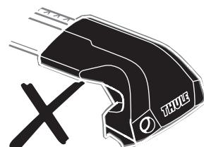
Do not use Thule Tents with any type of Thule Clamp or Thule Edge style roof racks as the high static weight may cause damage to your car's roof.
